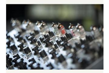
KERWAX Replica allows you to shape your very own sound character. The 12AX7 vacuum tubes that come standard can be replaced by alternative references like 12AY7 or 12AT7 to explore new possibilities.
